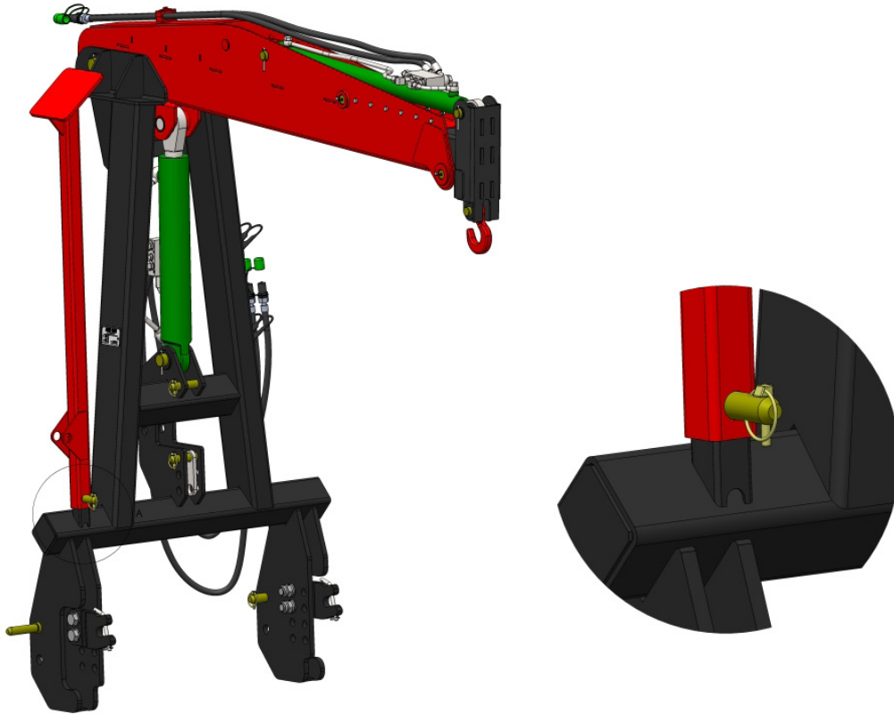
Fig. 7 Transport position of the loader: the support is on the frame and secured with the pin
